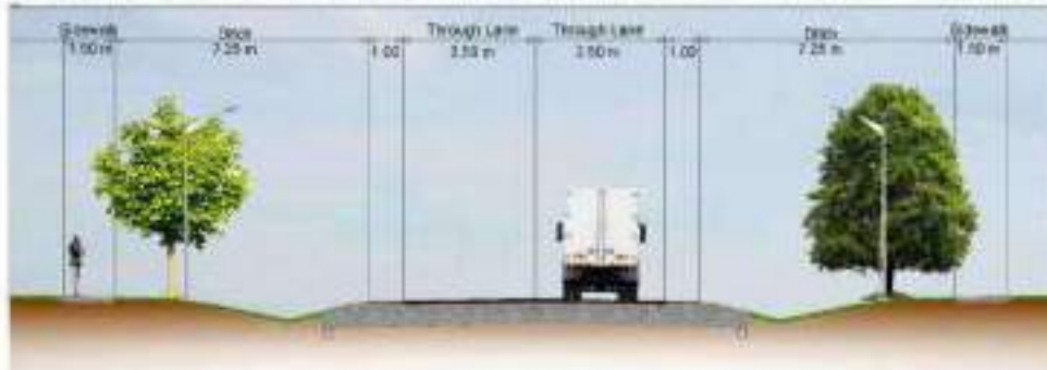
Clarkway Drive, EW Arterial to Countryside Drive - 30.0 m Right-of-Way, Separate AT Facilities
