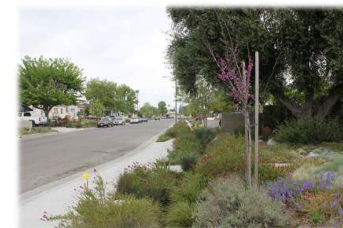
Example of roadside LID (Rain Garden)
