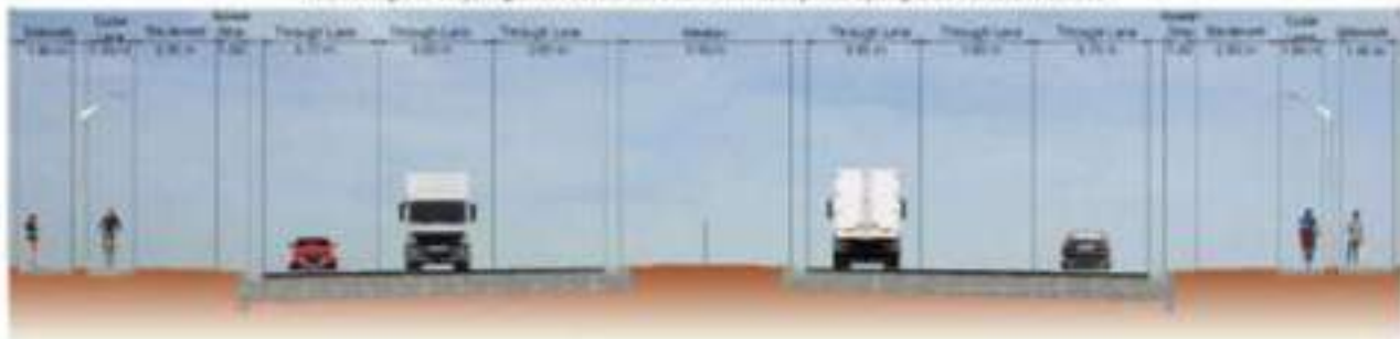
45.00 m Right-of-Way, Region of Peel Standard Lane Widths, Separate Cycling and Pedestrian Facilities
