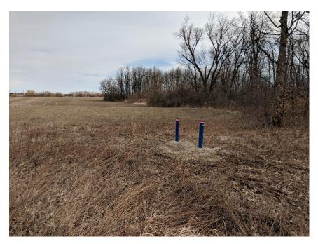
Photograph 1: Monitoring wells observed at the far west side of proposed alignment facing east.
