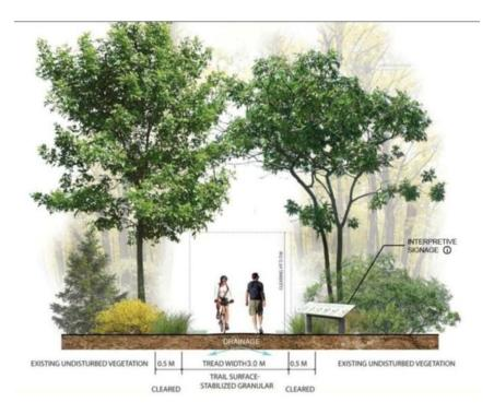
Figure 6: Example of granular trail cross-section
