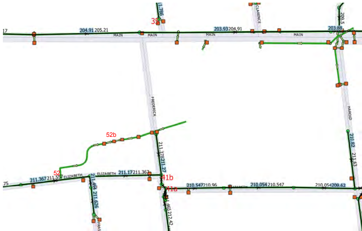
52 – Removed branch and routed catchments delineated from catchbasins to a downstream manhole where system would outlet.
