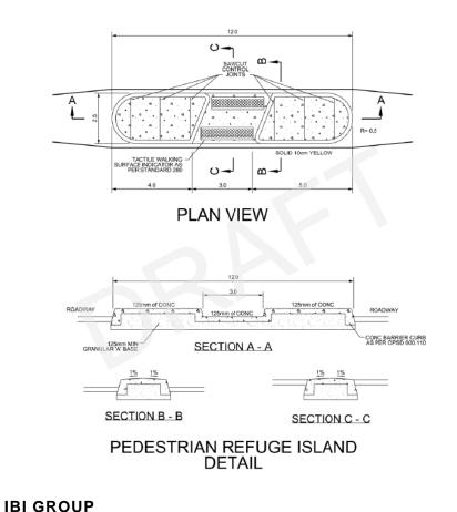
This example visualizes a new standard which may be used to provide a 'refuge island', in between the travel directions of a roadway.
