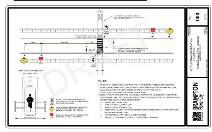
This example visualizes a new crossing standard, developed for unsignalized locations where a multi-use pathmeets a local road.
