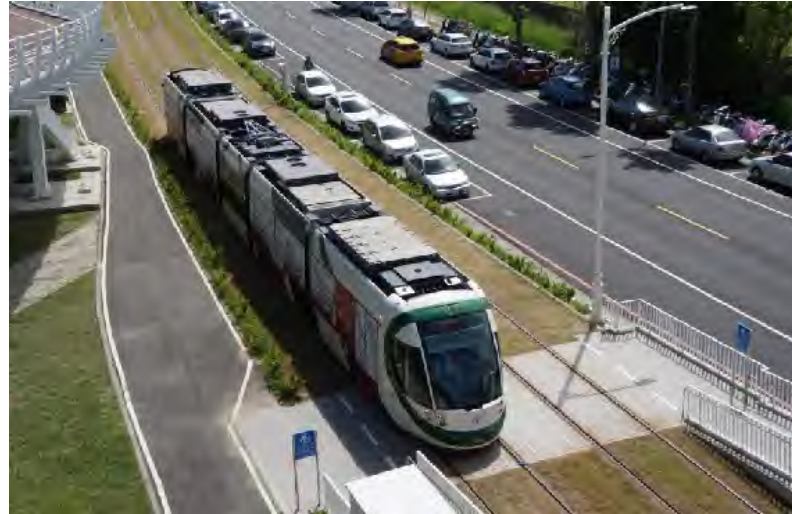
Catenary-Free Light Rail with Onboard Energy Storage and In-Station Charging (Kaohsiung, Taiwan)
