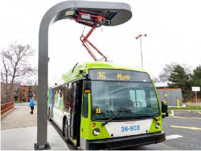
Electric Bus with End-of-Line Charging (Montreal, Quebec, Canada)
