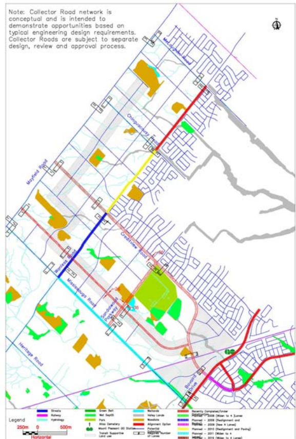
Exhibit 7.2 Alternatives 1 and 2 Required Lanes Mount Pleasant Secondary Plan Area Transportation Master Plan City of Brampton
