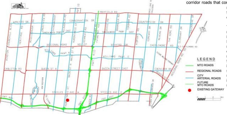
Figure 1.1 - City of Brampton Existing Arterial Corridor Plan
