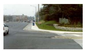
Figure 4.3.1 m - Arterial with sidewalk close to road edge and no street trees (Hurontario at Harold Street).
