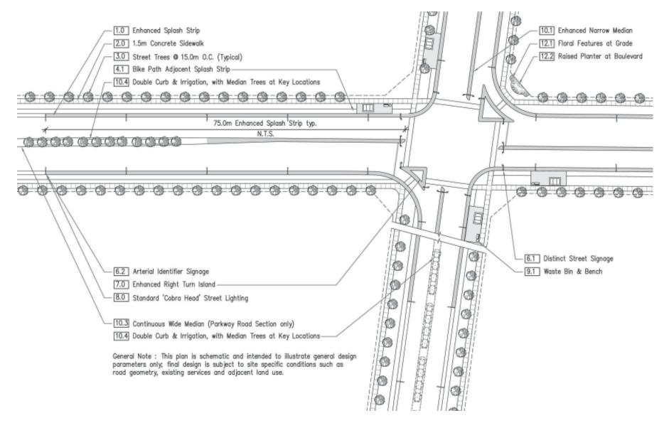
Figure 4.3.2 - Secondary Arterial Roads Concept Design
