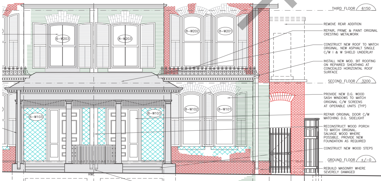
Figure 44. Conservation drawing of reconstruction. (Source: ERA)
