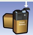
Cover the terminals on a 9-volt battery with electrical tape before disposing. If the terminals are accidentally connected, it can cause sparking.
