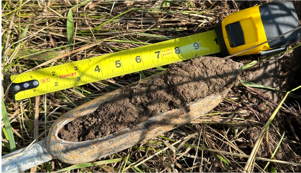
Photo 4-1: Typical dyke fill recovered during geotechnical investigation
