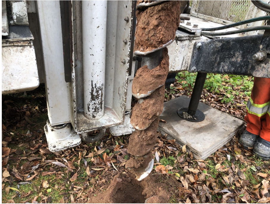
Photo 3-3: Auger sample taken during CPTu program
