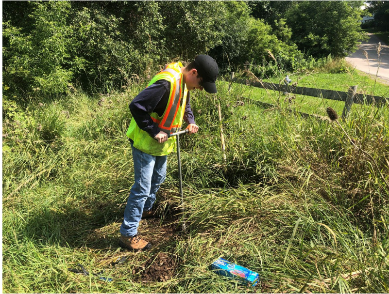
Photo 3-1: Hand auger investigation (Segment 1 – northern dyke section)
