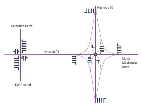
Figure 4: SPUI Interchange Lane Configuration
