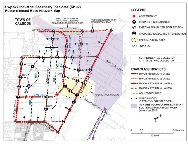
Figure 1: SP47 TMP-Recommended Road Network.
