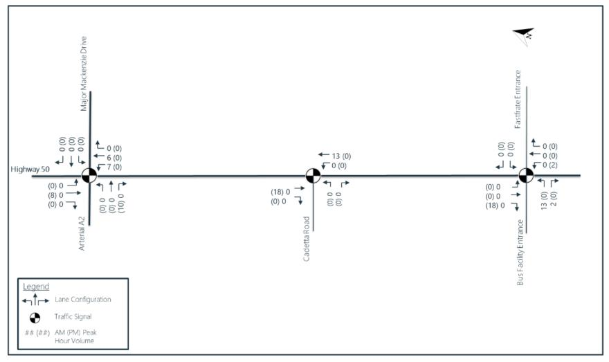
Figure 5: 2041 Bus Facility Site Trips (Buses)
