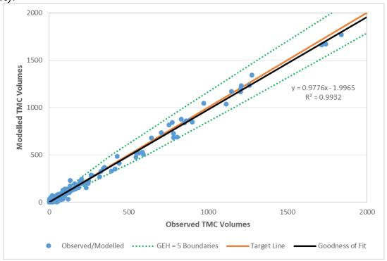
Figure 7: AM Peak Hour Modelled/Observed Volume Scatter Plot - Turning Movement
