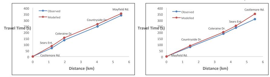
Figure 14: PM Peak - RR50 - NB (Left) and SB (Right) - Travel Time Comparison
