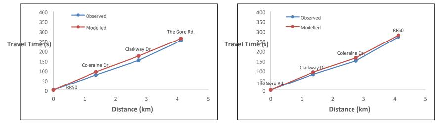
Figure 15: PM Peak - Mayfield Road - WB (Left) and EB (Right) - Travel Time Comparison
