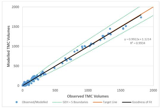
Figure 8: PM Peak Hour Modelled/Observed Volume Scatter Plot - Turning Movement
