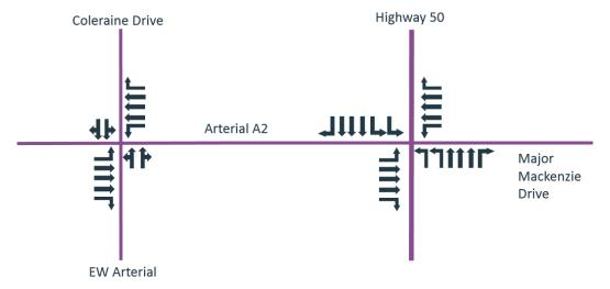
Figure 3: At Grade Intersection Lane Configuration
