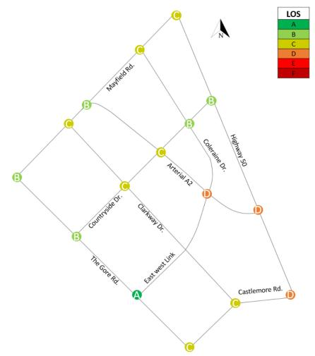
Figure 38: Signalized Intersections Level of Service - 2041 Realignment Alternative - AM Peak
