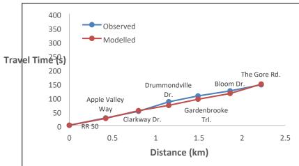
Figure 9: AM Peak Castlemore Road - EB (Left) and WB (Right) - Travel Time Comparison
