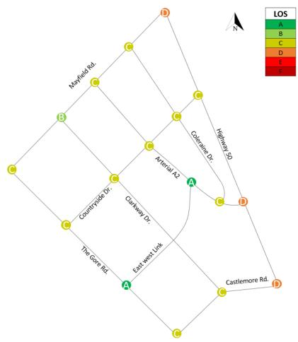
Figure 40: Signalized Intersections Level of Service - 2041 T-Intersection Alternative - AM Peak
