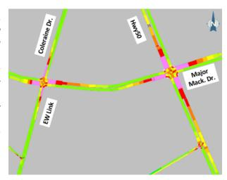
Figure 6: 2041 p.m. Peak Speed Plots for the At-Grade Intersection.
