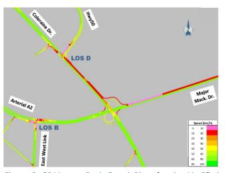
Figure 8: 2041 p.m. Peak Speed Plots for the Modified Parclo 'A' Interchange.
