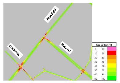
Figure 39: Zoom-in Speed Profile - 2041 T-Intersection Alternative - AM Peak
