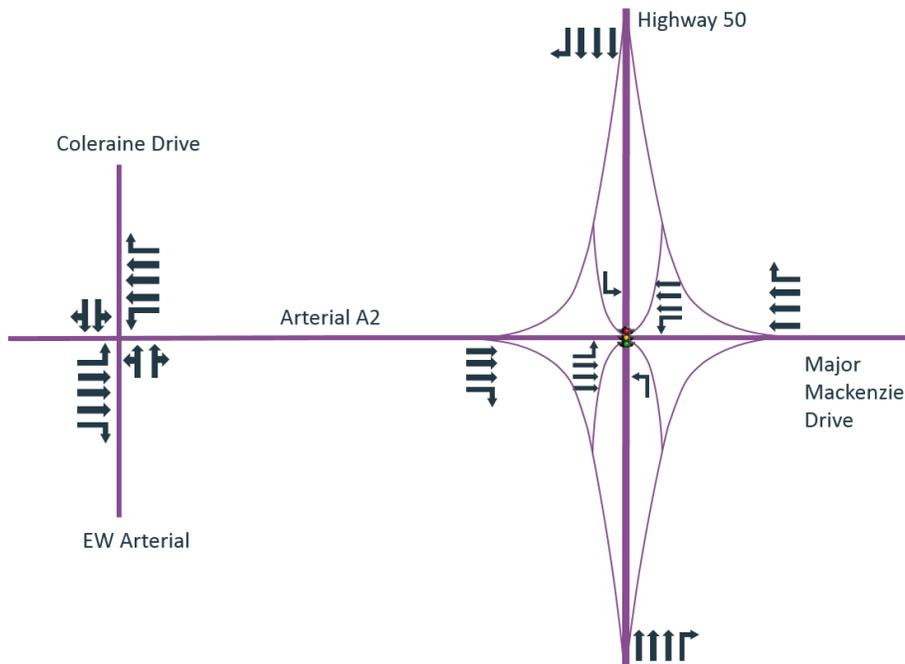
Figure 4: SPUI Interchange Lane Configuration
