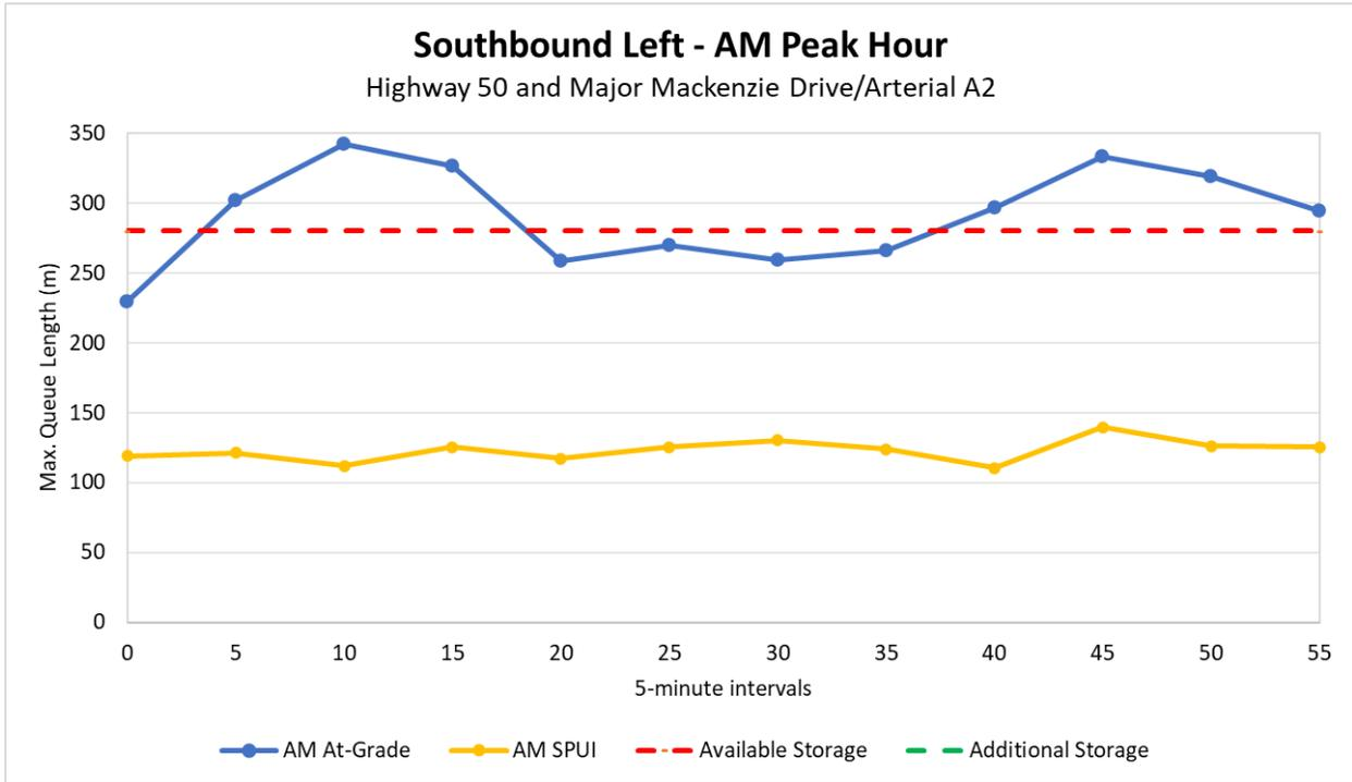
Figure 13: SB Left at SPUI (AM Peak Hour)
