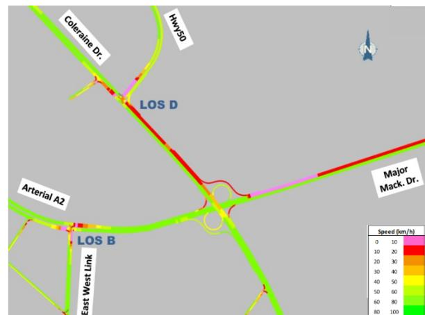
Figure 8: 2041 p.m. Peak Speed Plots for the Modified Parclo 'A' Interchange.
