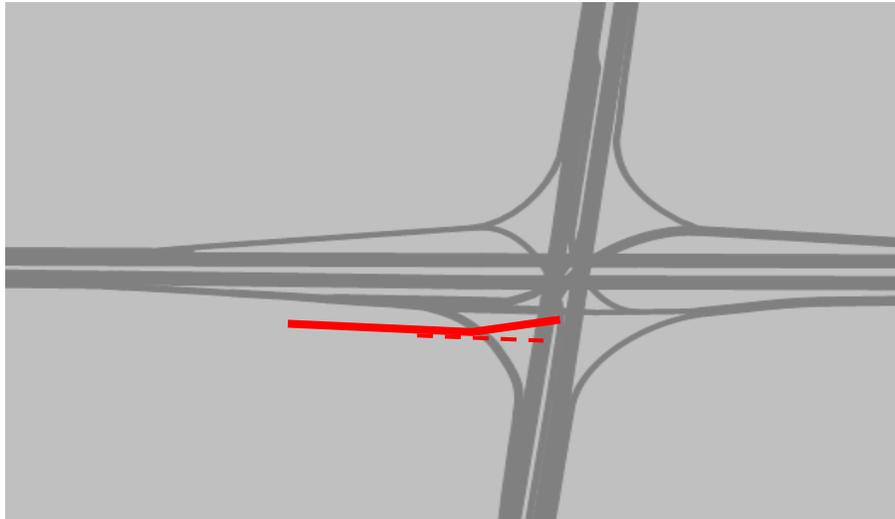
Figure 12: SB Left Queue Blocking Access to the Through Movement
