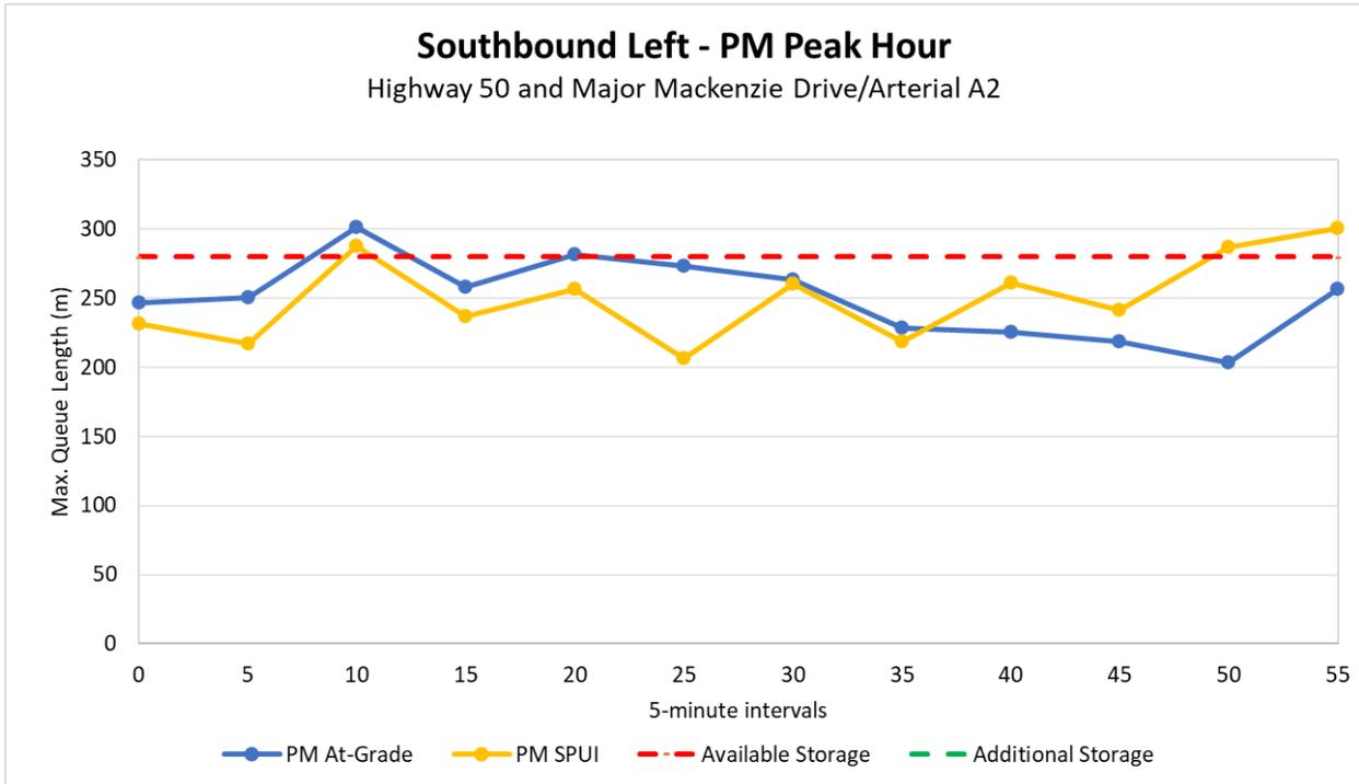
Figure 14: SB Left at SPUI (PM Peak Hour)
