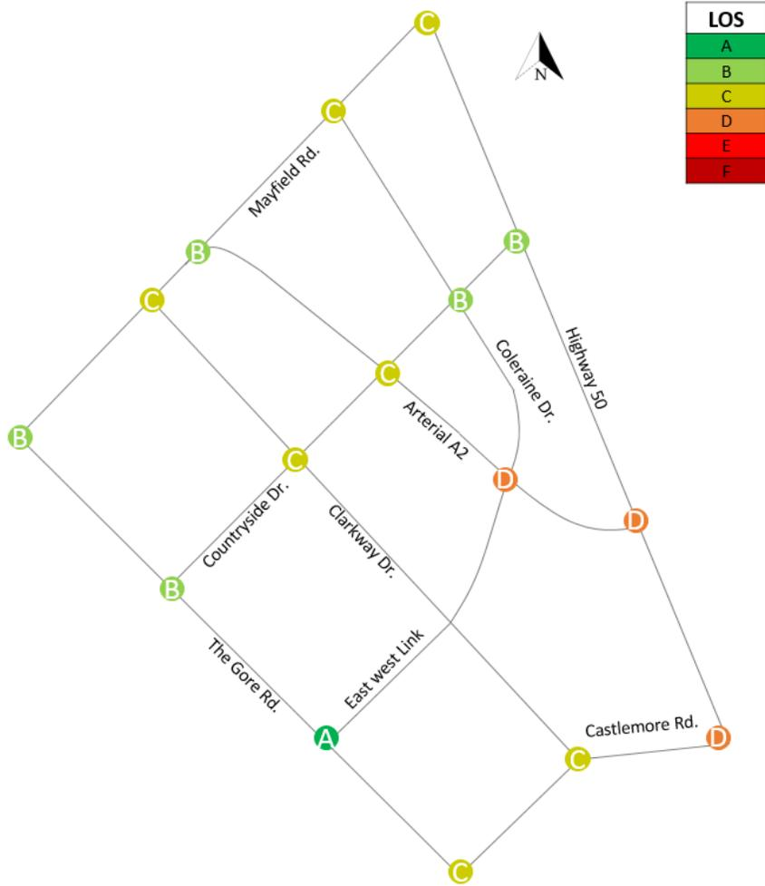
Figure 38: Signalized Intersections Level of Service - 2041 Realignment Alternative - AM Peak
