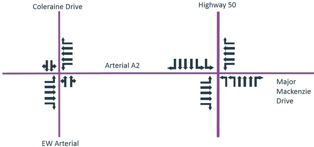
Figure 3: At Grade Intersection Lane Configuration
