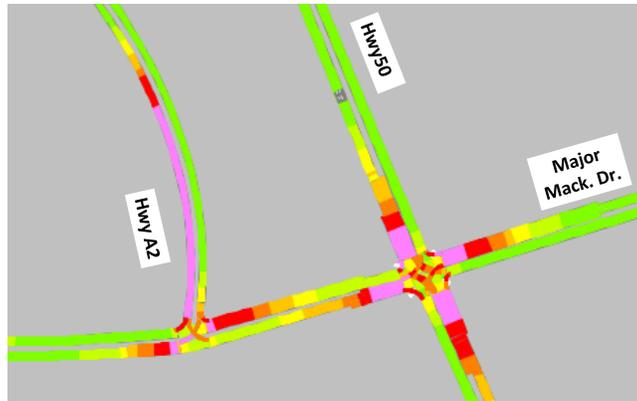
Figure 35: Speed Profile at Critical Intersections - 2041 PM Peak
