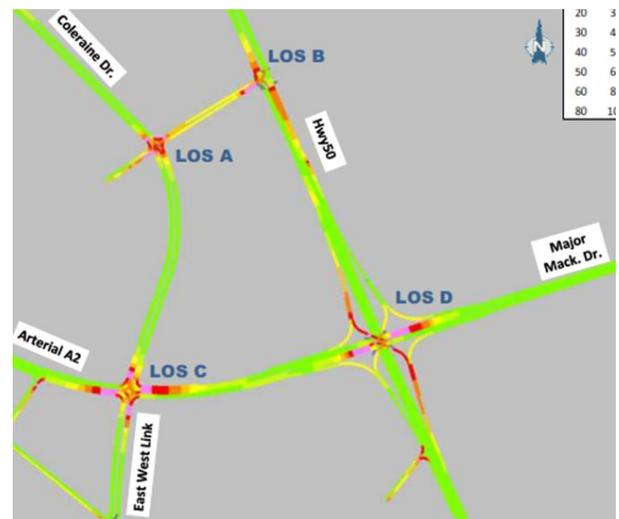
Figure 7: 2041 p.m. Peak Speed Plots for the SPUI Grade-Separation.
