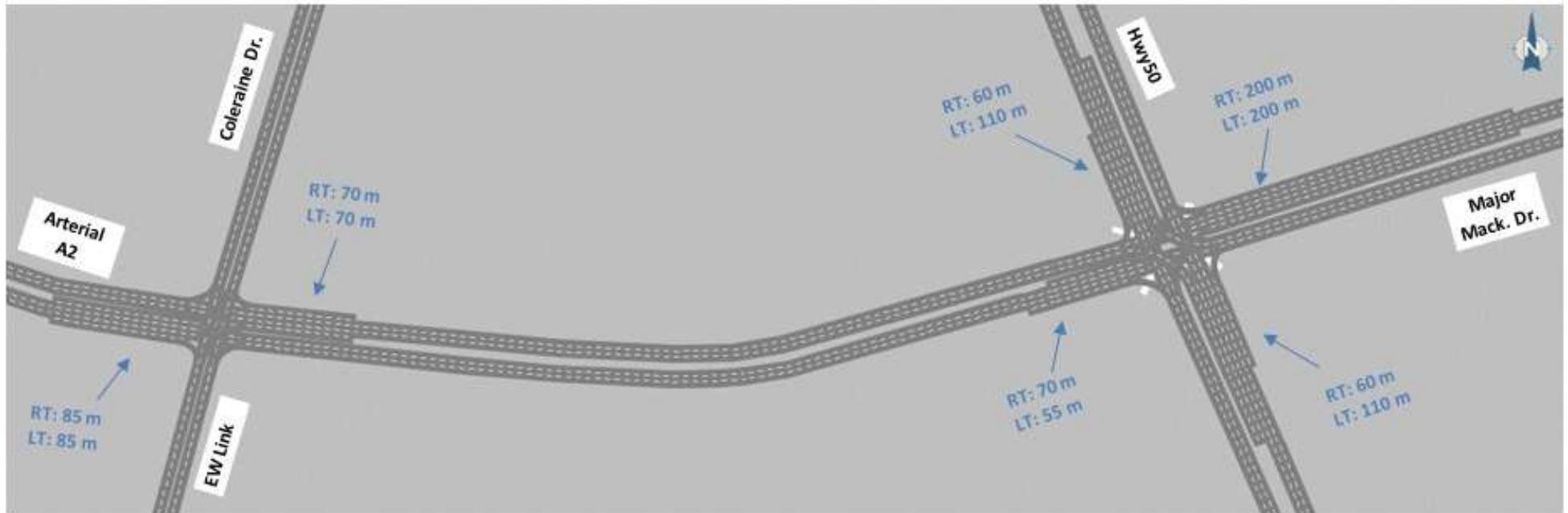
**Critical Intersection Storage Length – 2041 Alternative T-Intersection at Arterial A2/Mayfield Rd.**
