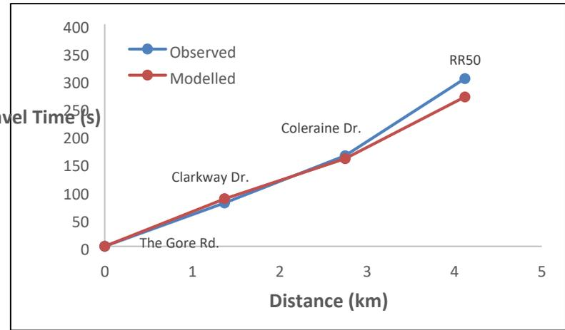
Figure 11: AM Peak - Mayfield - WB (Left) and EB (Right) - Travel Time Comparison
