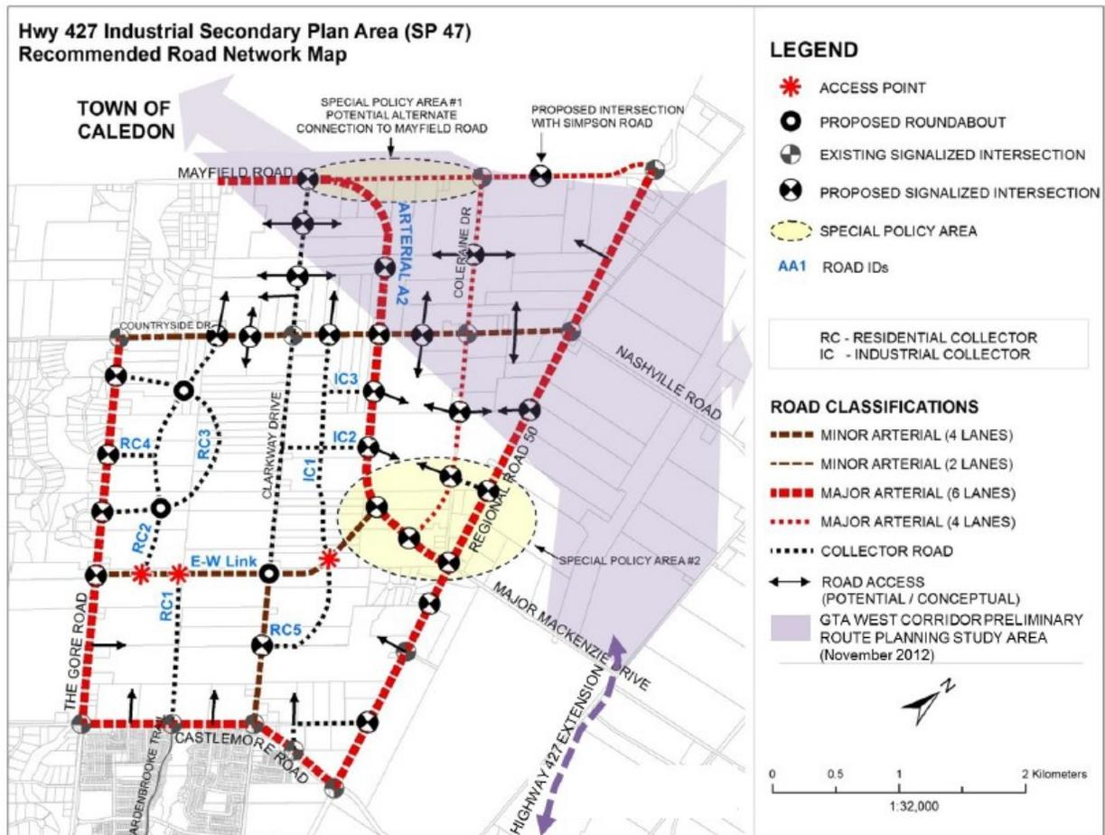
Figure 17: SP47 TMP Recommended Road Network
