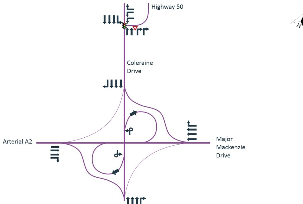
Figure 5: Modified Parclo A-Type Interchange New Lane Configuration
