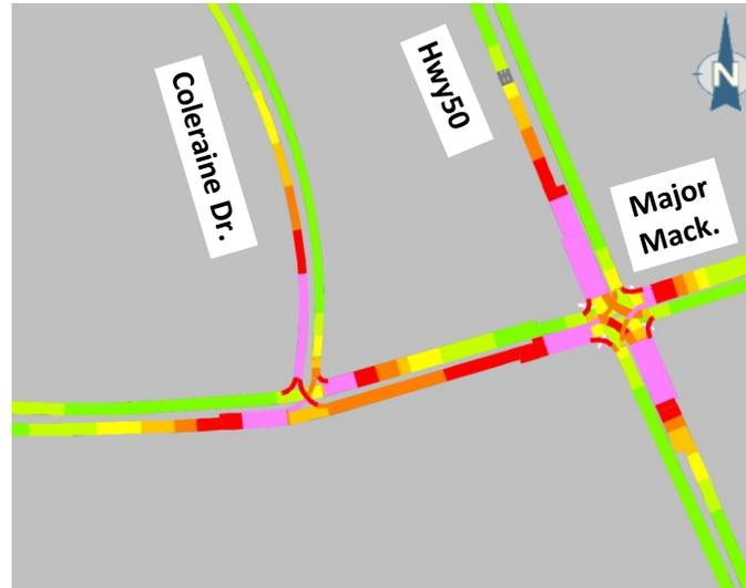
Figure 31: Speed Profile at Critical Intersections
