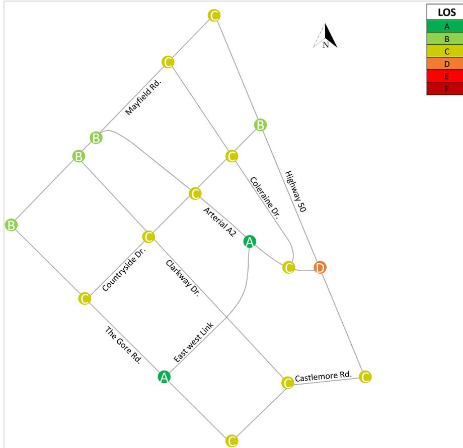
Figure 29: Signalized Intersections Level of Service - 2031 PM Peak
