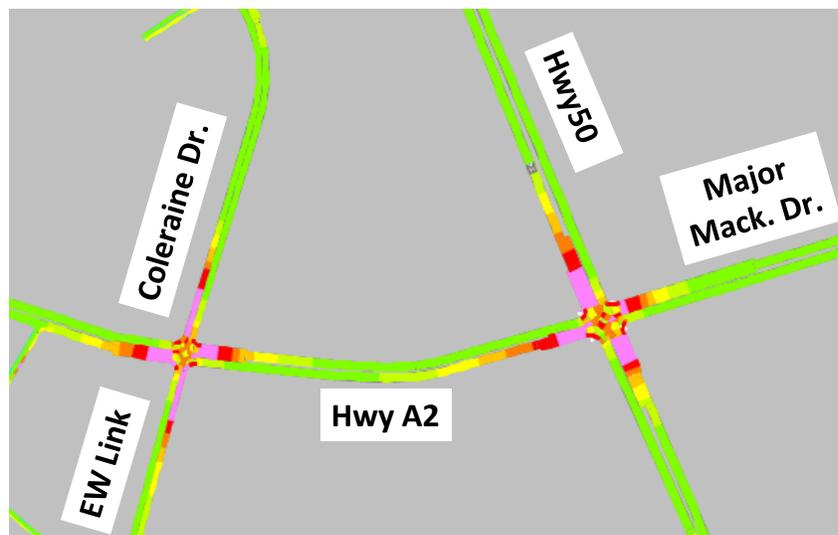
Figure 37: Speed Profile - 2041 Realignment Alternative - AM Peak
