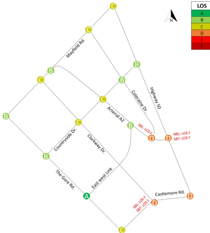
Figure 33: Signalized Intersections Level of Service - 2041 AM Peak
