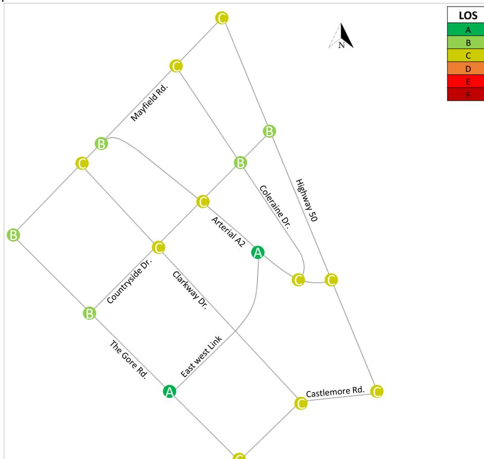
Figure 26: Signalized Intersections Level of Service - 2031 AM Peak
