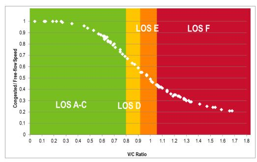
Figure 2-1: Relationship between Congested/Posted Speed Ratio and V/C Ratio
