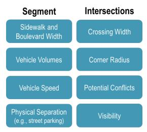
Figure 2-5: Inputs for Pedestrian LOS
