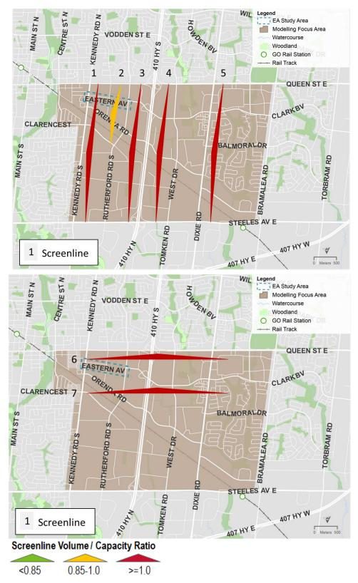
Figure 4-2: Screenline V/C Ratio, 2041 Do Nothing (EA) Peak Hour, Peak Direction
