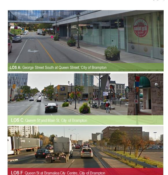
Figure 2-6: Examples of Pedestrian Level of Service
