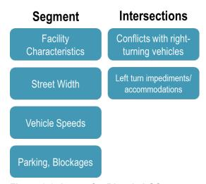
Figure 2-3: Inputs for Bicycle LOS
