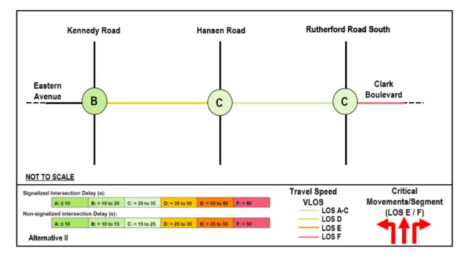
Figure 5-3. 2041 PM Alternative 3 (Do Nothing TR) VLOS Diagram
