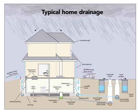
This diagram illustrates features that make up a typical home drainage system for residential homes.
