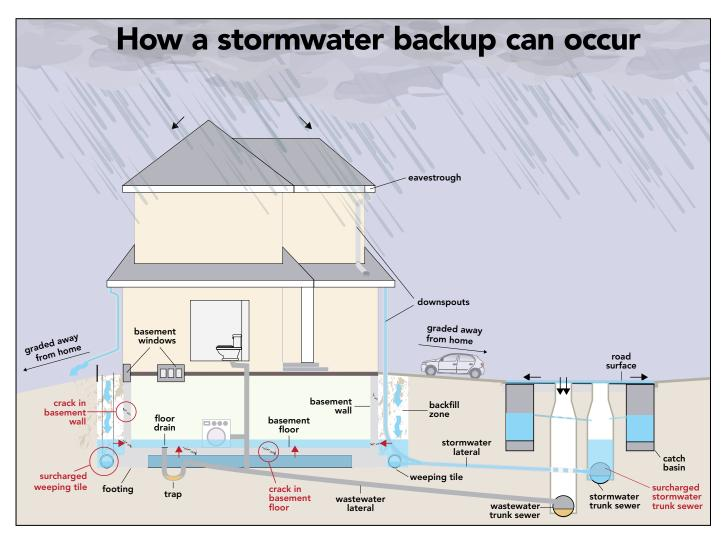
This diagram illustrates problems with typical home drainage features that could lead to a wastewater back up in a residential home.
