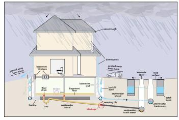
This diagram illustrates how a blockage in the wastewater lateral can lead to basement flooding.
