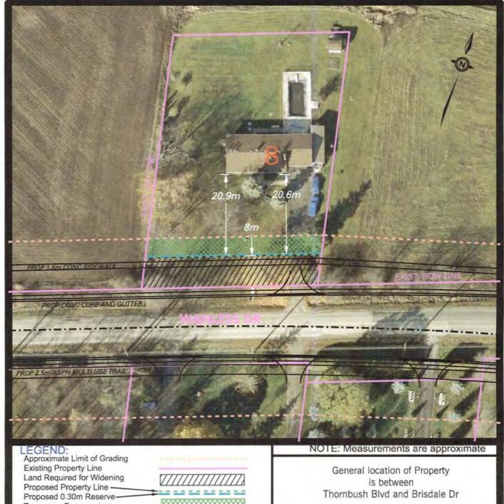
Temporary Easement Temporary Easement Limit Line Permanent Easement Permanent Easement Limit Line
