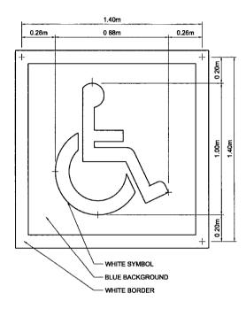
2. The following diagram illustrates the location of the pavement markings within a typical accessible parking space.
