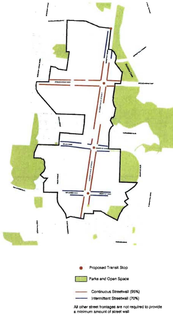
Figure 8.3.3 Brampton Gateway Continuous Street Frontage Map
