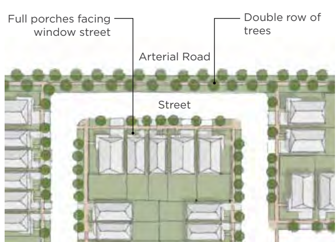
Window Street Condition
