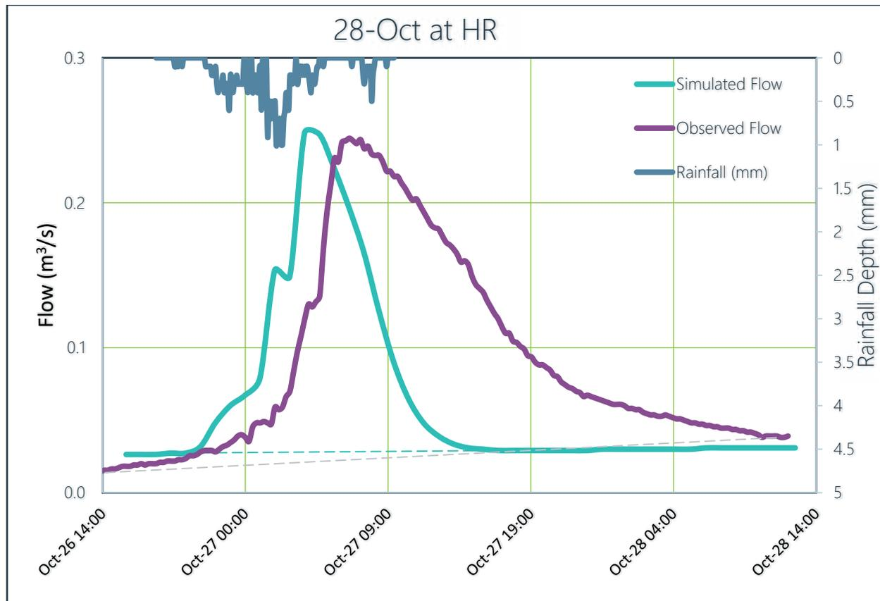
**Figure Hydro 6. CRT2 (Upstream of Bovaird Drive) October 28, 2019 Observed Flow Hydrograph and Rainfall Hyetograph**
