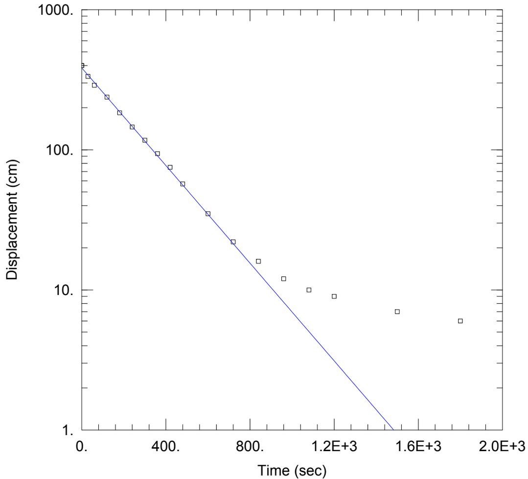
HYDRAULIC CONDUCTIVITY TEST AT MW7D
