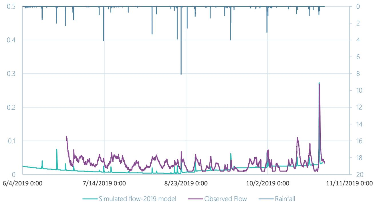
**Figure Hydro 5. CRT2 (Upstream of Bovaird Drive) 2019 Observed Flow Hydrograph and Rainfall Hyetograph**
