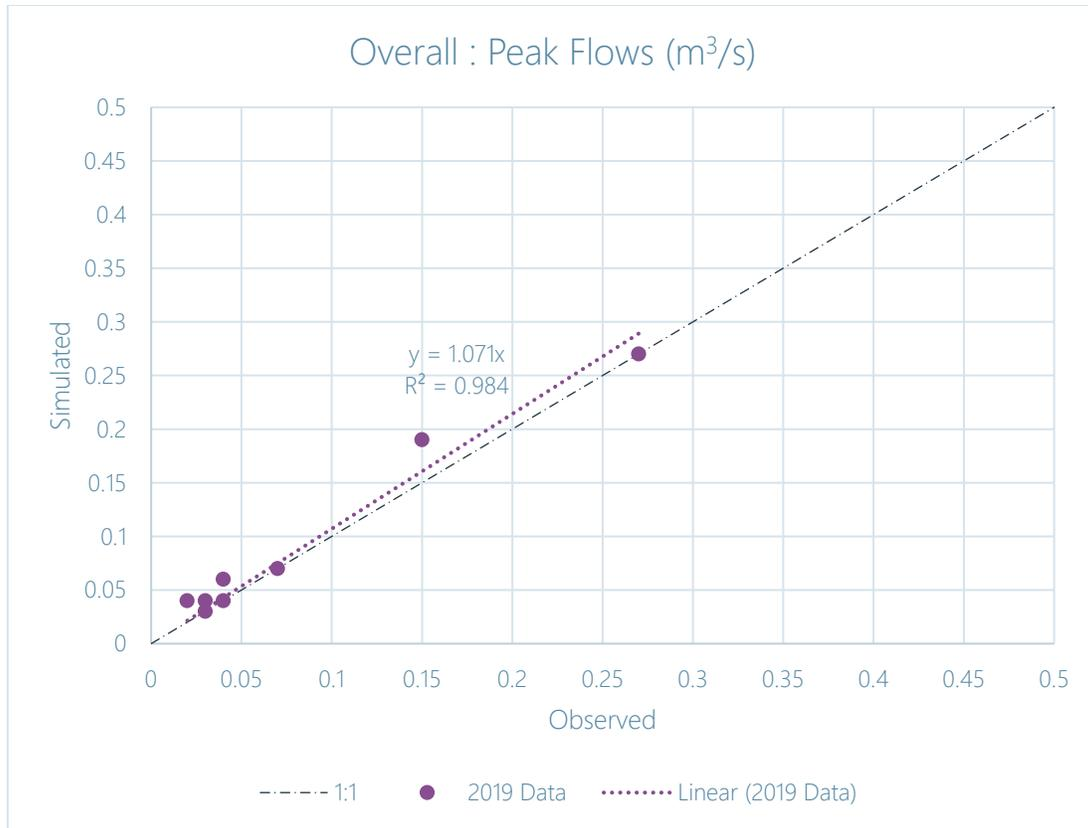
**Figure Hydro 7. CRT2 (Both Gauges) Observed versus Simulated Peak Flows (m<sup>3</sup>/s)**
