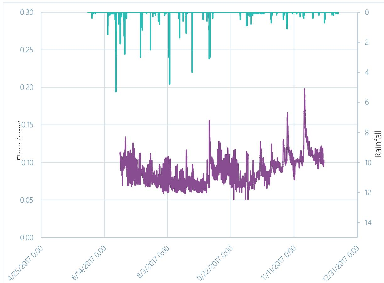
**Figure Hydro 4. Observed Flow Hydrograph and Rainfall Hyetograph**
