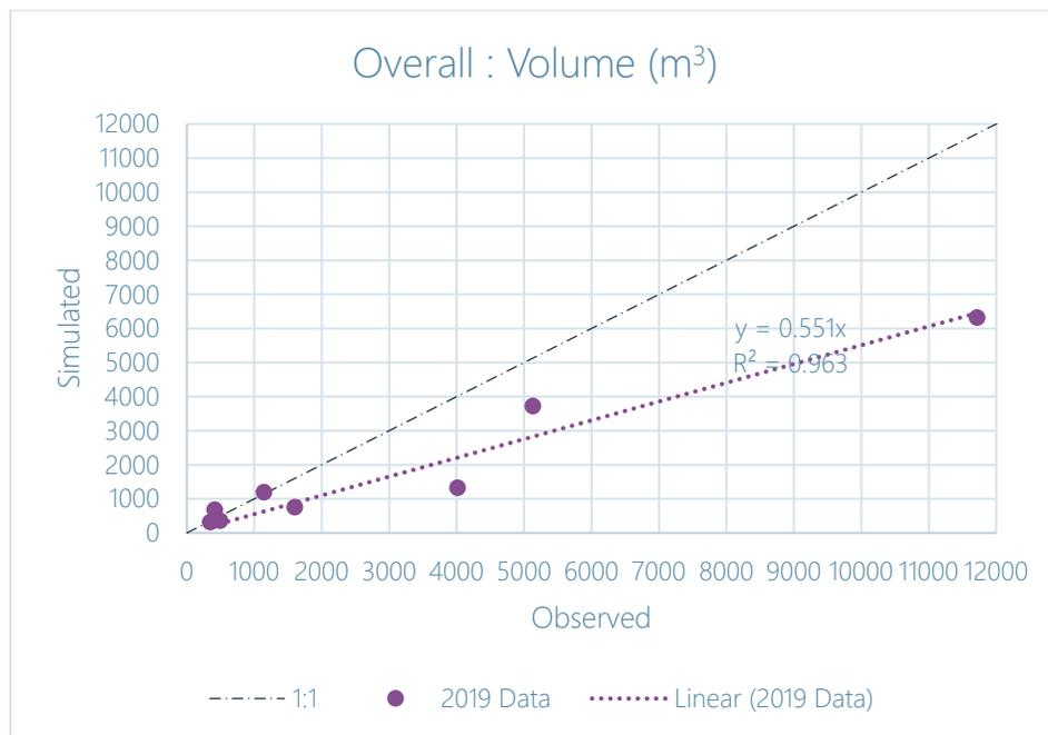
**Figure Hydro 8. (Both Gauges) Observed versus Simulated Runoff Volumes (m<sup>3</sup>)**
