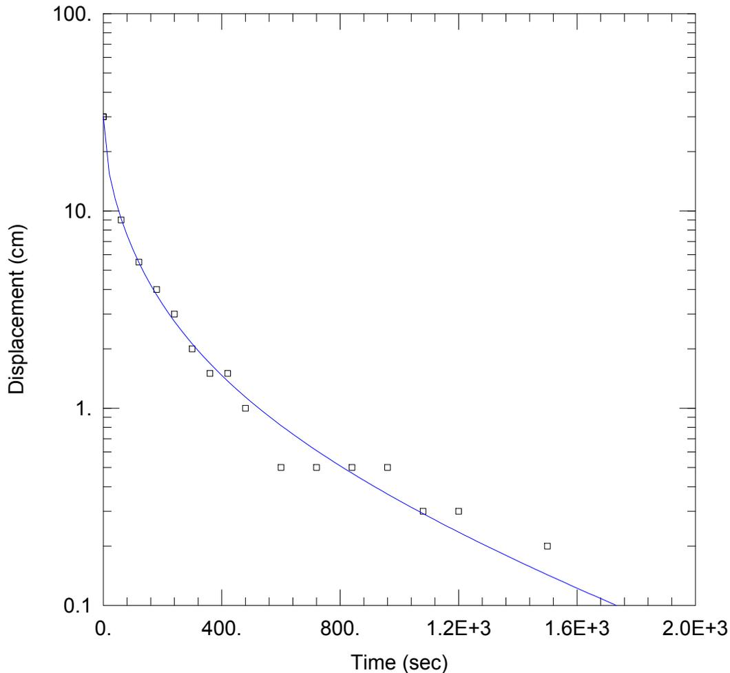
HYDRAULIC CONDUCTIVITY TEST AT MW8
