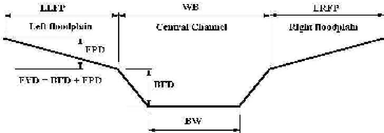
**Figure Hydro 1. Channel Cross-Sections Definitions used for Cross-Sections**
