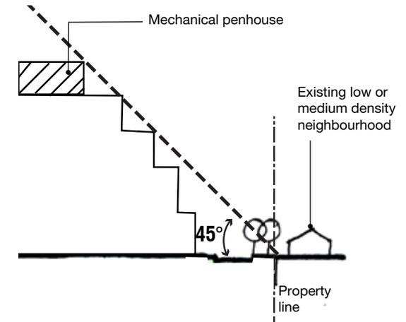
Mechanical penthouses must conform to the angular plane controls.
