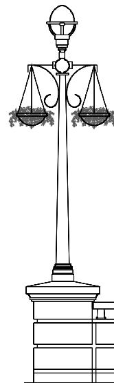
*Figure 5.4.1b Bridge End Pier Elevation with light standard and floral baskets.*
