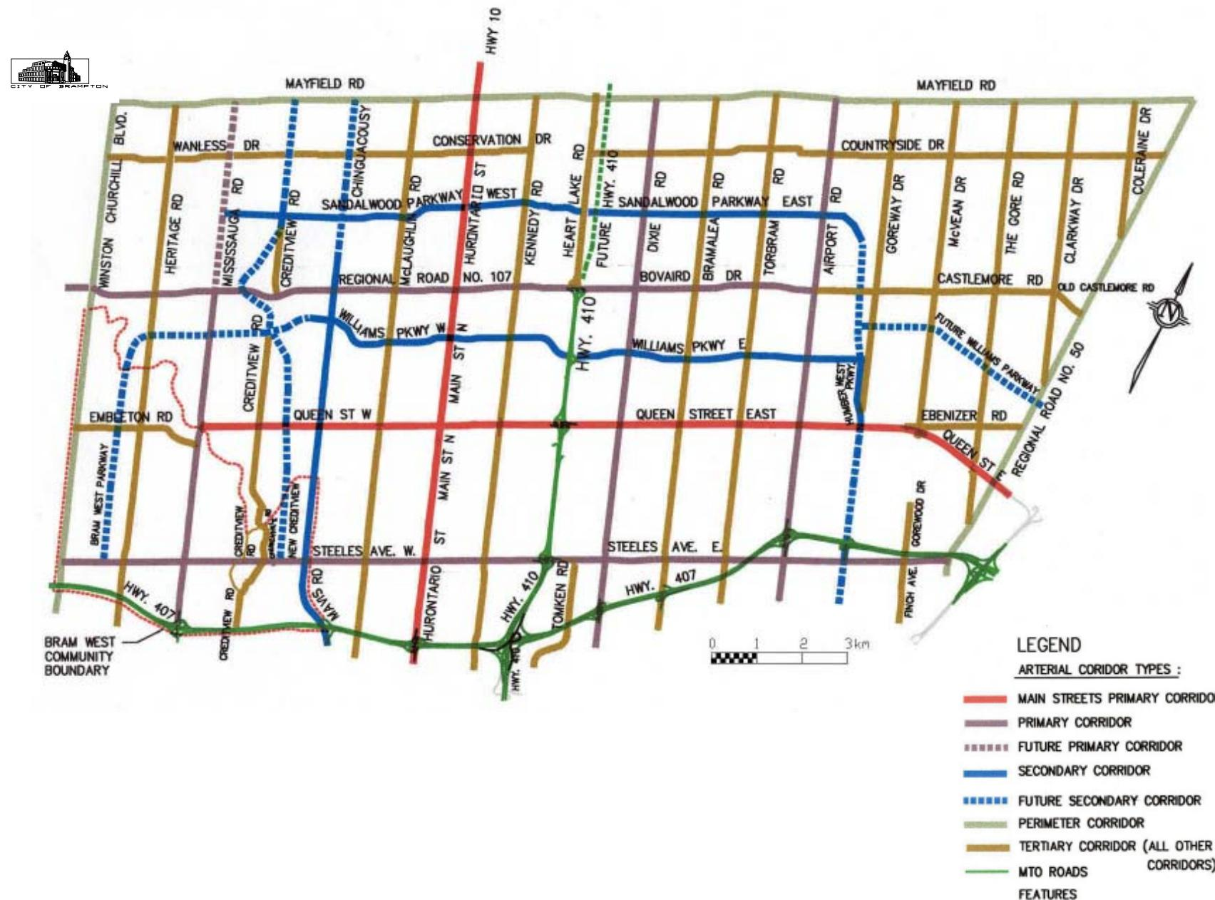
Figure B.1 - Arterial Corridor Hierarchy Mapping
