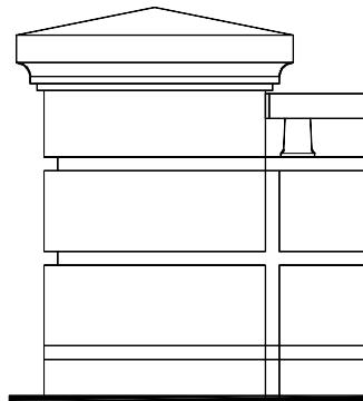
*Figure 5.4.1a Bridge End Pier Elevation*
