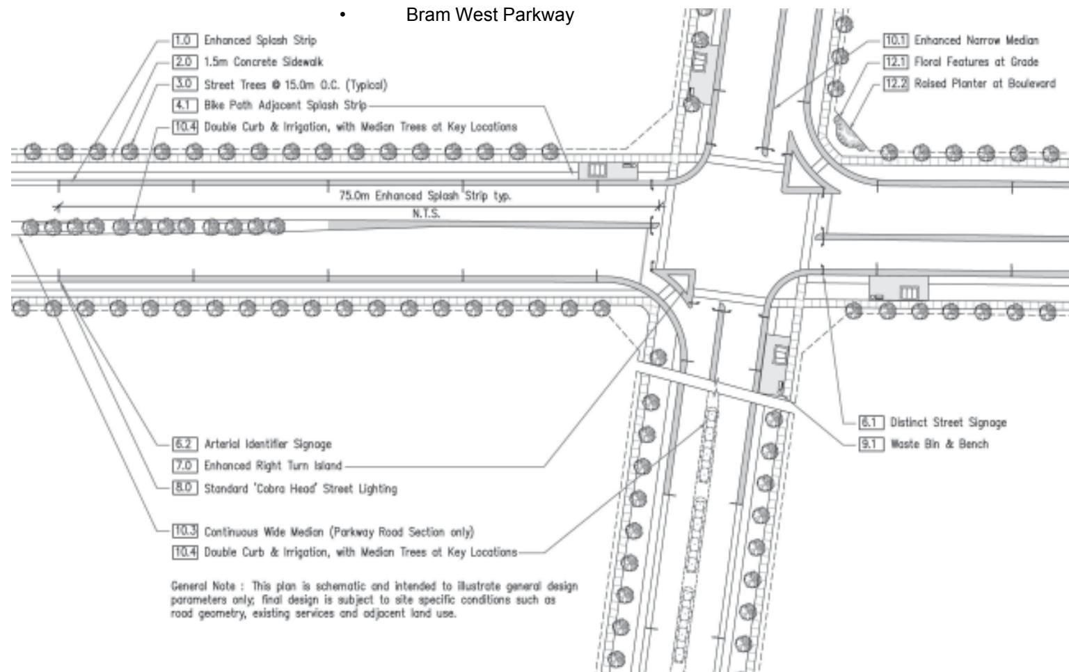
Figure 5.2.3 Enhancements for Secondary Arterial Roads.
