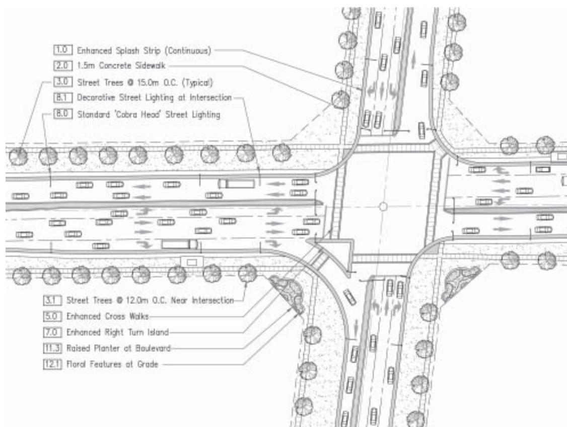
Figure 5.6.2a Plan Detail at Median (Regional Road 107 / Bovaird Drive & Mississauga Road)
