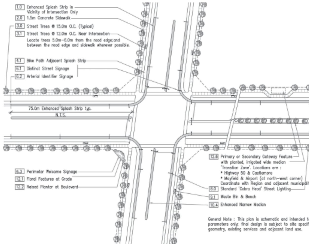
Figure 5.2.4 Enhancements for Perimeter Arterial Roads.
