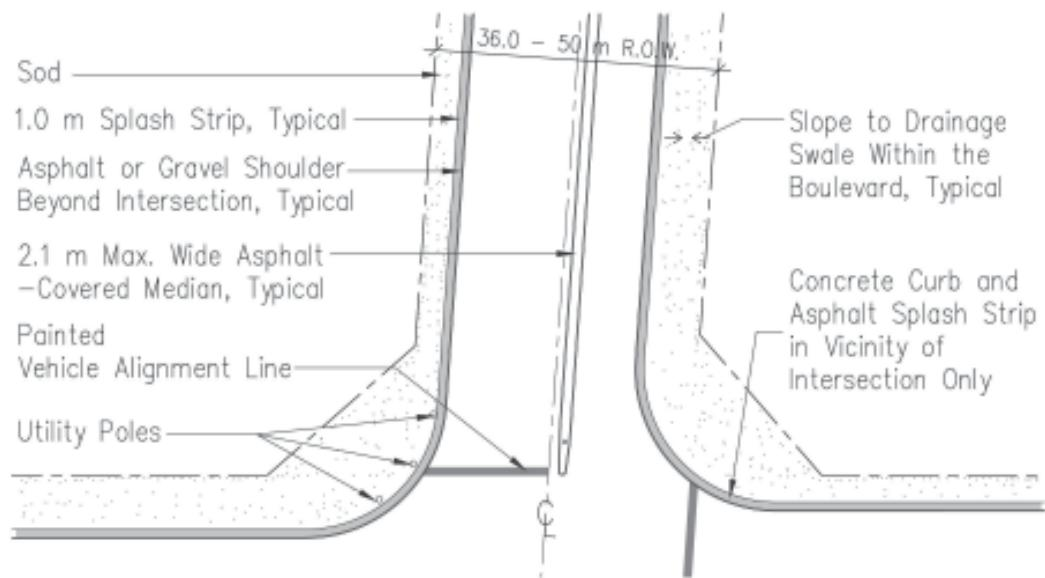
Figure 4.1.1 g- Plan of Arterial Intersection (Rural Road Section)
