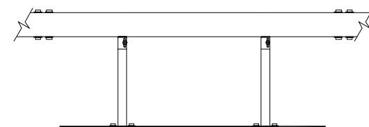
*Figure 5.4.2 Guide Rail Elevation*
