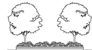
**11.7** Raised planters with irrigation; design, materials and location coordinated with accompanying feature elements located within the adjacent boulevard. (eg. Hurontario Street Anchor and/or Primary Gateway + Transition zone).
