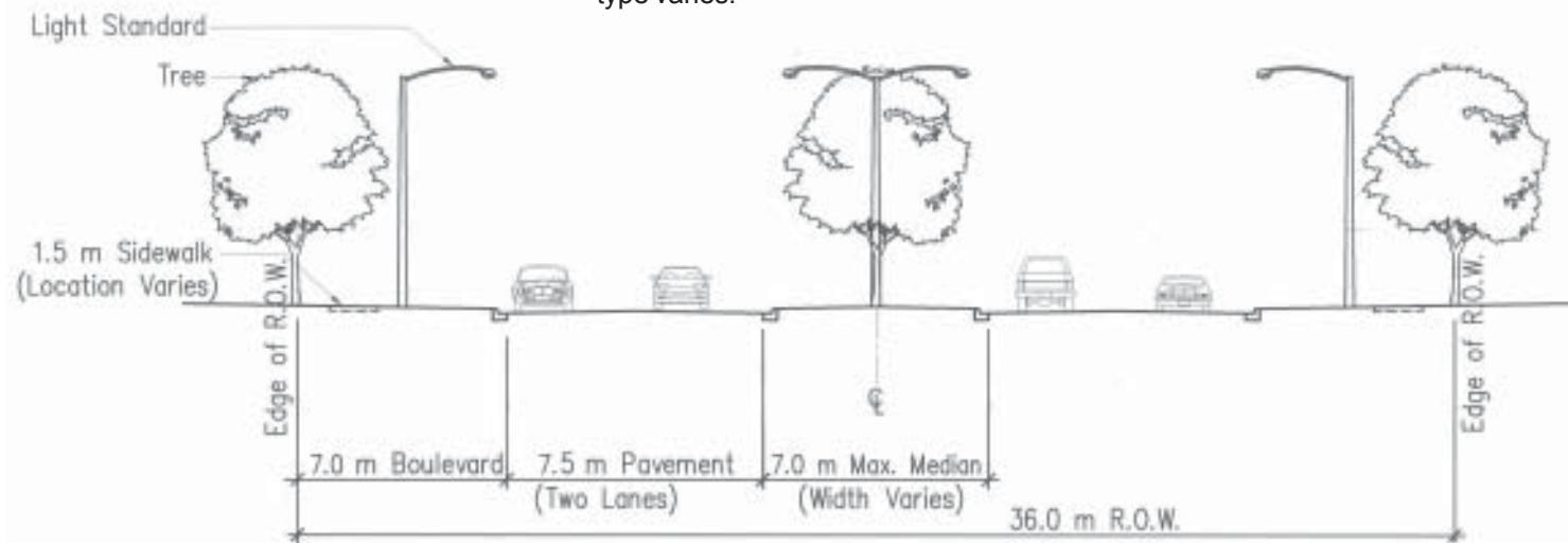
Figure 4.1.2 a - Existing Parkway Prototype Section
