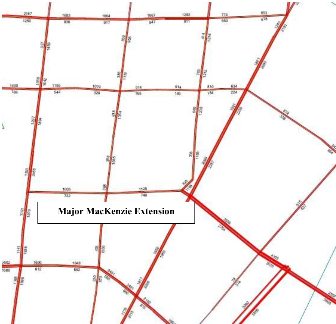
Exhibit 8-3: Auto Volume Plot, 2009 YP BATS Recommended Alternative - No Major MacKenzie Drive - Mayfield Road Link
