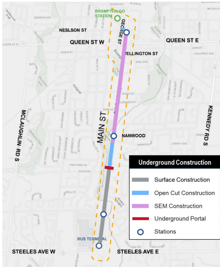
Figure 7-1: Underground Options Construction
