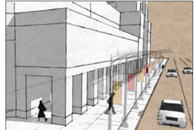
Arcade can be used to make the development attractive, interesting and comfortable for pedestrians.
