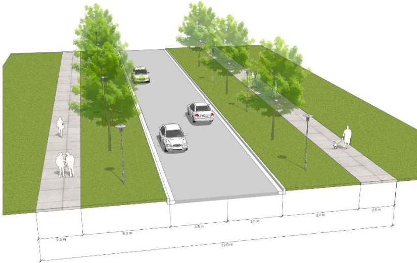
Figure A12: Remote Street without On-Street Parking
